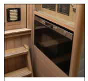
MICROWAVE A stainless steel microwave is placed at chest height in the aft locker by the rear steps.
