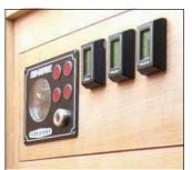
**CONTROL PANEL** The engine control panel is set into the port locker, along with digital gauges for water, diesel and toilet tank levels.
