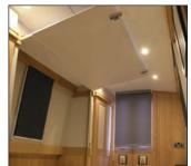
ROOF BLIND When making up the cross bed, the upper flap of cupboard acts as a blind for the rooflight above.
